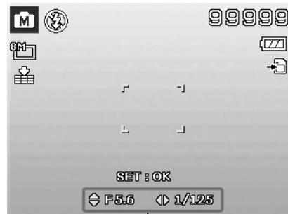
Displays the aperture and shutter speed value
