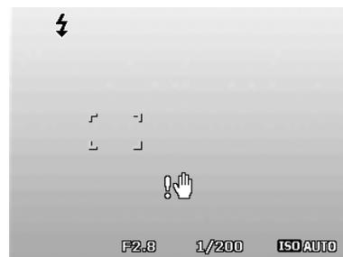
When the shake warning icon
